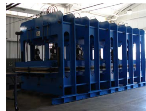
26' x 8' Heated Platen Press for Foam & Beam Constructed Enclosures
