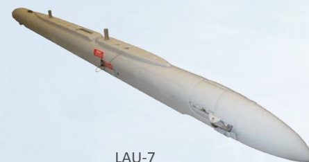
LAU-7 Sidewinder Missile Launcher
