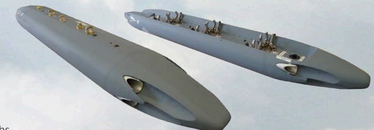
SUU-20 Bomb Dispenser and Rocket Launcher
