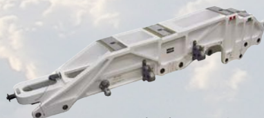
Low in Bay (LIB) Internal Weapons Bay Adapter
