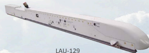
LAU-129 AMRAAM Missile Launcher
