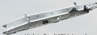
High in Bay (HIB) Internal Weapons Bay Adapter
