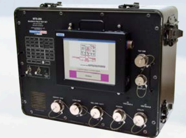
MTS-206 Maverick/Hellfire System Test Set
