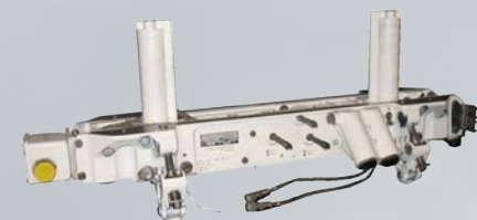
BRU-56 B-1B 30-inch Ejector Rack
