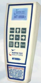
MT1888 Series Laser Source Simulator
